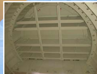
747F Barrier Beams
